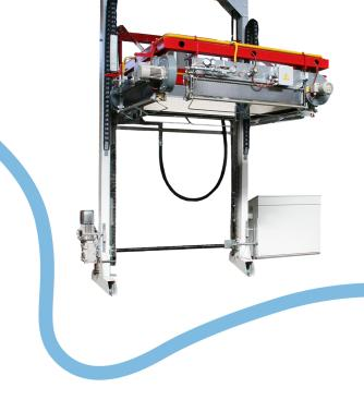
The OMS FT-55 Pallet Shrink Hooding Machine is a free-standing gas-fired shrink ring machine which applies heat to shrink-film bags (aka shrink pallet covers) normally applied manually to packs upstream of the machine.
